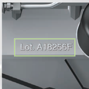
Presence inspection of marked characters
